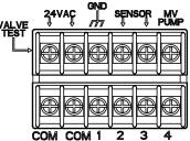
VALVE TEST – Use this terminal to test a valve for proper function.
